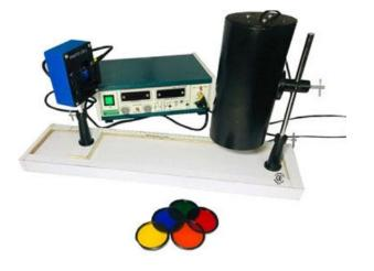
**AGN-388 Description:** Experimental Set-up has been designed specifically for determination of Planck's constant by Vacuum type Photo Cell with three ilters. The experimental set-up is absolutely self contained and require no other apparatus. Photo Cell with three ilters. Practical experience on this set up carries great educative value for Science and Engineering Students.
