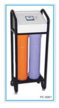
Capacity 50 Ltr/Hr, Consists of two plastic column charged with high exchange capacity Cation & Anion resins. Conductivity Meter Provided
